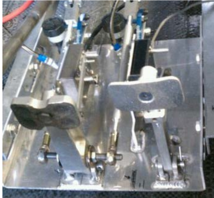
Figure 3.3.3 – Solar car's New Pedal Cluster
