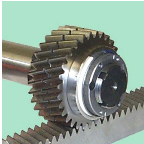
Figure 4.2.2 – Rack and Pinion Gear
