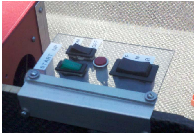
Figure 9.1.2 – Three switches used by the driver to start the car
