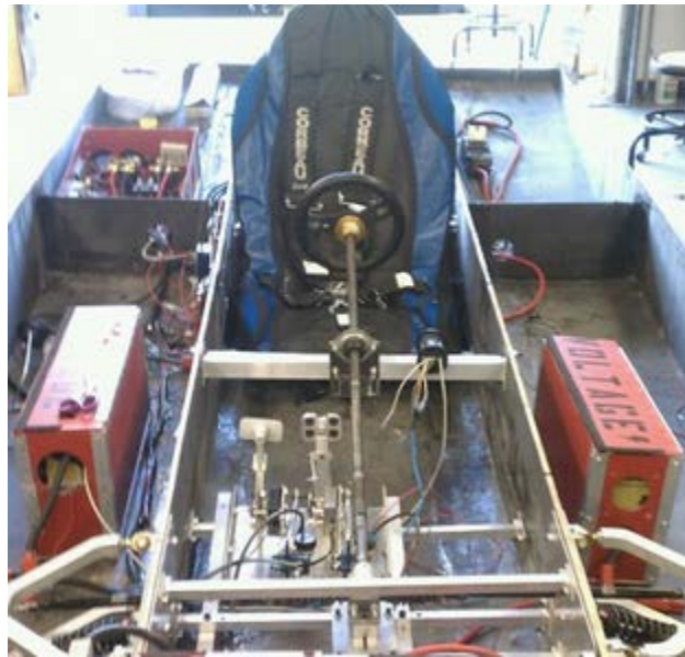
Figure 3.1.2.2: Steering Column Mounted in Car
