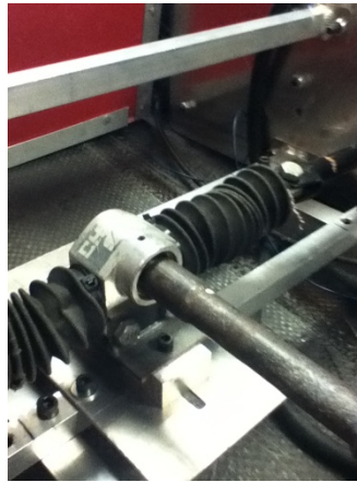
Figure 3.2.2 – Rack and Pinion Gear (Rack and Pinion)
