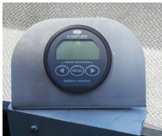
Figure 9.1.3 – The state of charge display for the driver
