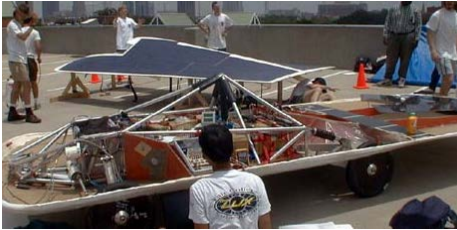
Figure 3.1.4---Aluminum Frame with Outer Shell (Cyber, 1999)
