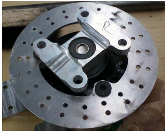
Figure 3.3.8 – Brake Rotor Mounted on Spindle
